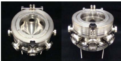
Photo Credit: Matthew Post, co-author Figure 2: The NREL sensor test chamber with viewing port on a load-lock lid and 8 side ports for pneumatic and electrical feedthroughs.
